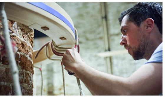
Inspired by traditional woodworking, the connections of the upper ring are made with modern hand and power tools. Precision is key: the more surface contact in the joint, the stronger it is, and this accuracy is achieved entirely by hand and eye.
